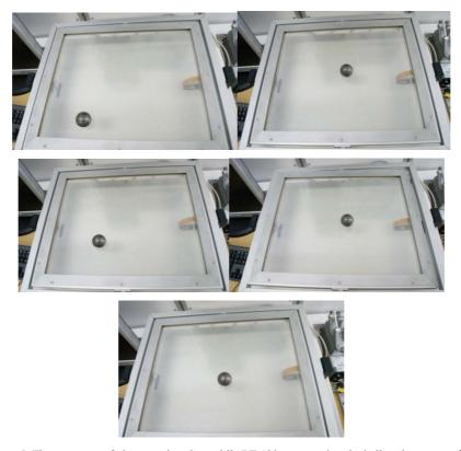
Figure 5. The sequence of photographs taken while RT 123 was moving the ball to the centre of the plate. The pictures were taken in the laboratory of Warsaw University of Technology, the faculty of Automatic Control and Robotics.
