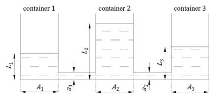
Figure 3. Three containers scenario, where  $L_1$ ,  $L_2$ ,  $L_3$  denote levels of water in corresponding containers,  $A_1$ ,  $A_2$ ,  $A_3$  denote their cross-sectional areas, and  $a_1$ ,  $a_2$  denote the cross-sectional areas of corresponding pipes.
